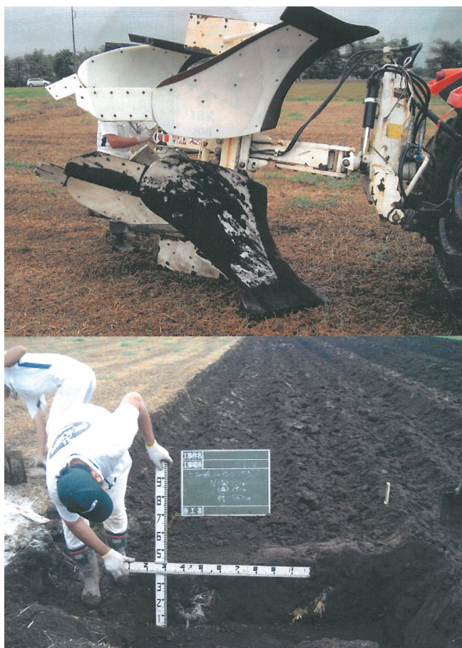
Fig. 1. Deep-plowing method with soil horizons mixing (Japan)
