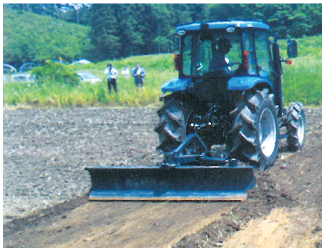
Fig. 2. Upper contaminated ground layer removal (Japan)
